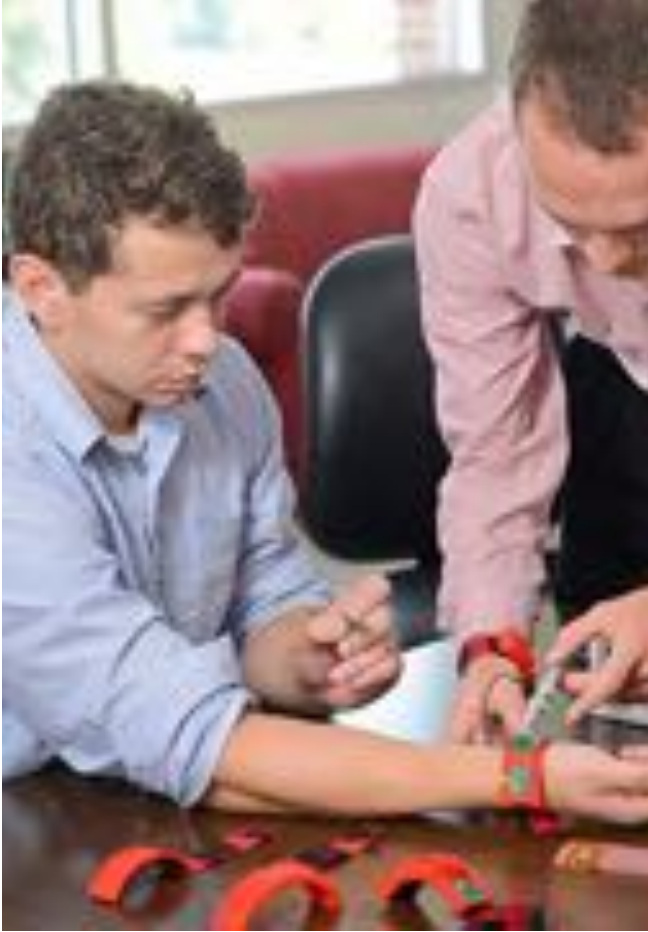
Dieffenderfer, left, and undergraduate Eric Beppler work on the SoliBand, a solar-powered health monitoring device that is worn on the wrist.
